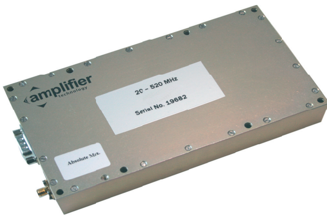
ATL broadband power amplifier that delivers saturated output power of 125W for frequencies of 20MHz to 520MHz. The amplifier is designed as a 'commercial of the shelf' product (COTS), providing high output powers with good overall efficiency.
